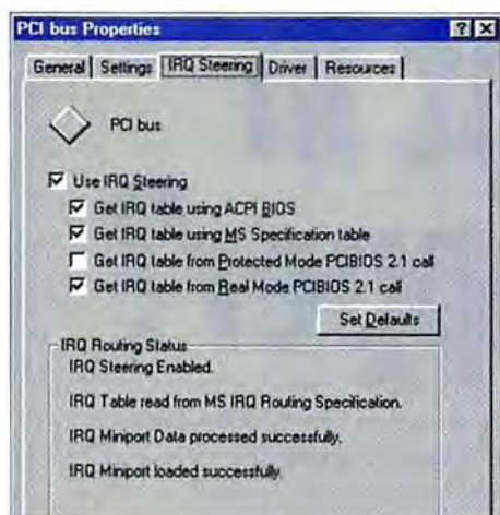
FIGURE 2: BY ENABLING IRQ Steering in Device Manager, you can let PCI cards share an IRQ.
