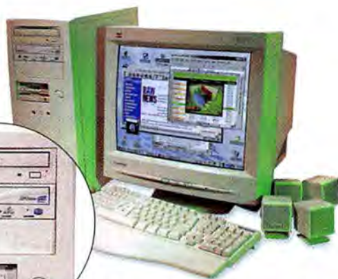
BURN, ZIP, OR JUST WATCH: Along with a hard drive, Axis Systems' Orion 100A DVD gives you several storage options, including a CD-RW drive, an Iomega Zip 100 drive, and a DVD-ROM drive.
