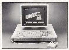
The AT&T UNIX\* PC A multi-user, multi-tasking processor with integrated voice and data communications functions.
